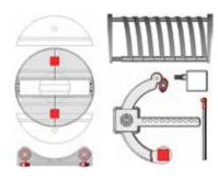
First a concept with 6 motors, and now just one, which normally is turning the table in microwave ovens. Very simple mechanics as in every car engine: camshaft.
